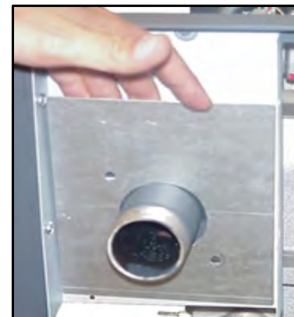
Figure 8: Removing End Plates
